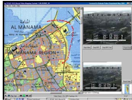
An RTGIS screenshot, with map, aircraft trail and position displayed on the left and a live video feed and grabbed frame on the right.
