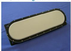
The Navtech **NTS-HE102** GPS Compass provides TRUE heading from the GPS satellites. By simultaneous and coincident constellation tracking, two receivers with common processing derive the local GPS position, differential GPS corrections and heading with respect to True (geographic) North.
