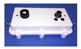
The Navtech NTS-HS220 GNSS Compass Module provides TRUE heading from the GPS, GALILEO, GLONASS, & BeiDou, satellites. By simultaneous and coincident constellation tracking, two receivers with common processing derive the local position, differential GNSS corrections and heading with respect to True (geographic) North using signals from two antennas on a 0.3 to 5 meters a base line. Position accuracy using SBAS is better than 1 meter.
