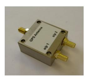
The Navtech Systems miniature GPS Splitter NTS-SMA enables two GPS receivers to share a single antenna. Using a combined low noise amplifier and power by-pass circuitry, the GPS antenna will supply amplified GPS signals via a Wilkinson splitter to one or both receivers connected to the outputs. Antenna power supplied by either GPS receiver is by-passed to the antenna, to enable active antennas to be used as the primary signal source in any GPS installation.
